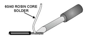
Figure 2-27.—Tinning wire with a soldering iron.
