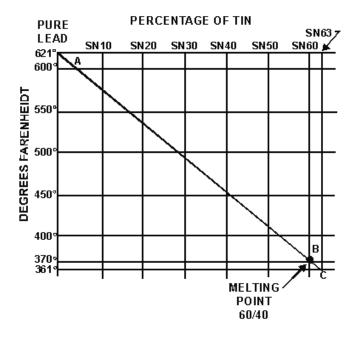
Figure 2-35.—Tin-lead fusion diagram.
