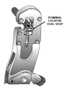
Figure 2-21.—Crimping tool with terminal lug inserted.
