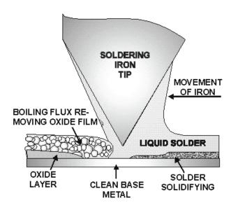
Figure 2-36.—Action of flux.
