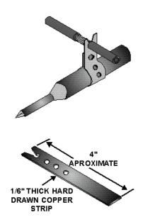
Figure 2-4.—Locally made hot-blade stripper.
