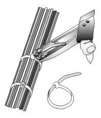
Figure 2-50.—Installing self-clinching cable straps.
