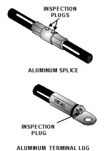
Figure 2-17.—Aluminum terminal lug and splice.
