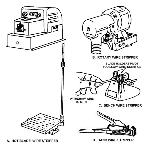
Figure 2-1.—Typical wire-stripping tools.
