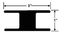
Figure 2-40.—Lacing shuttle.
