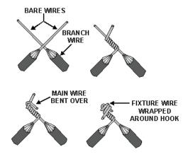
Figure 2-8.—Fixture joint.
