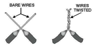
**Fixture Joint**—When conductors of different sizes are to be spliced, such as fixture wires to a branch circuit, the fixture joint is used.
