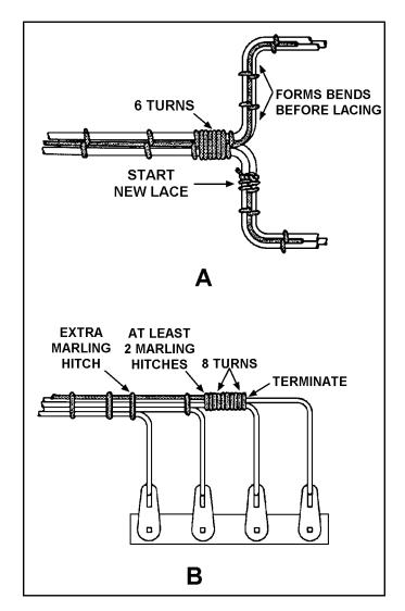
Figure 2-42.—Lacing branches and breakouts.
