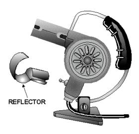
Figure 2-15.—Typical hot-air gun.
