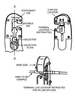
Figure 2-24.—Locating splice in crimping tool.
