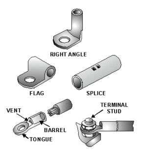
Figure 2-11.—Noninsulated terminal lugs and splices.
