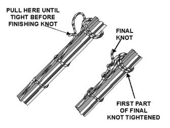
Figure 2-45.—Alternate method of terminating the lace.
