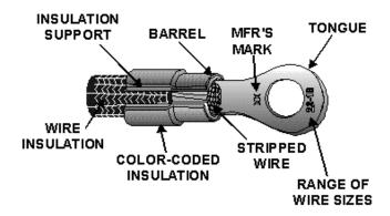
Figure 2-19.—Preinsulated straight copper terminal lug.
