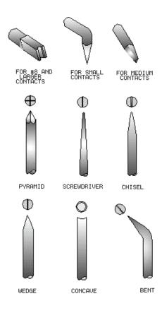
Figure 2-29.—Soldering iron tip shapes.
