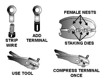
Figure 2-12.—Crimping small copper uninsulated terminals.
