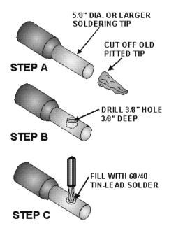
Figure 2-26.—Alternate dip-tinning method.
