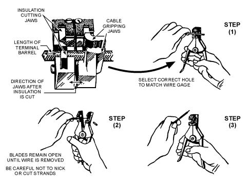
Figure 2-2.—Stripping wire with a hand stripper.
