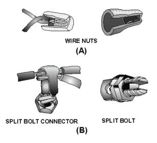
Figure 2-10.—Wire nut and split bolt splices.
