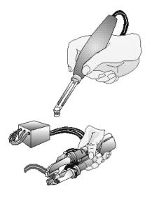
Figure 2-32.—Resistance soldering set
