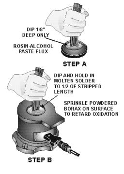
Figure 2-25.—Dip-tinning In a solder pot.
