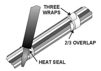
Figure 2-52.—Securing wire bundles in high-temperature areas.
