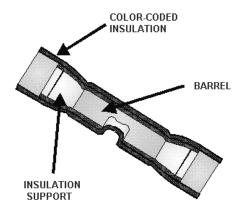
Figure 2-23.—Preinsulated copper splice.
