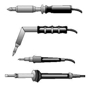
Figure 2-28.—Types of hand soldering Irons.
