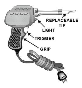
Figure 2-31.—Soldering gun.
