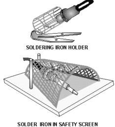
Figure 2-38.—Soldering iron safety devices.
