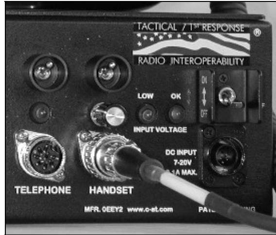
FIGURE 22: TELEPHONE INTERFACE JACK
