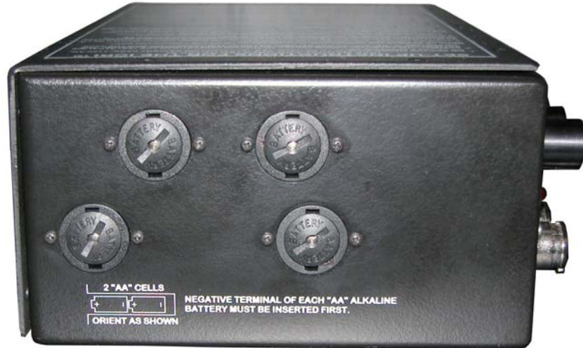
FIGURE 10: ICRI WITH INTERNAL BATTERIES
