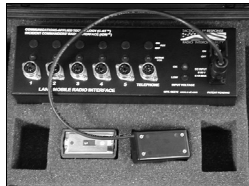
FIGURE 9: BATTERY ATTACHMENT TO ICRI (VIEW 2)
