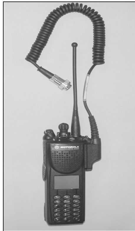
FIGURE 15: RADIO WITH ICRI CABLE ATTACHED
