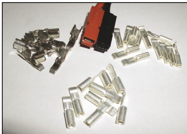
Figure 3 — On the left are 45 A contacts; notice the open ends that must be crimped. The standard 30 A size in the center or the smaller 15 A size on the right may be crimped or soldered.
