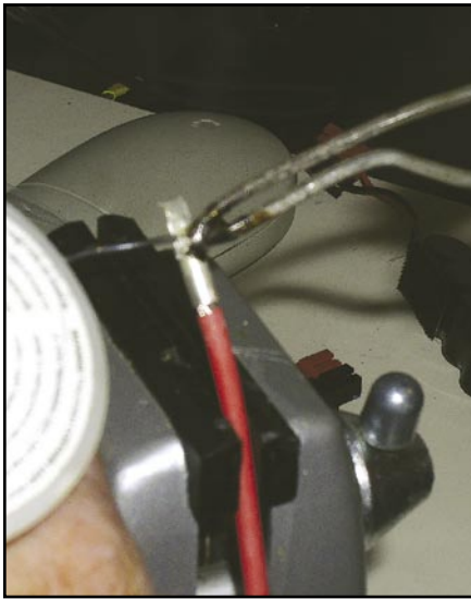
Figure 4 — To solder a Powerpole connector, place the tip of your soldering iron against the body, right at the end of the wire inside the connector. Melt a small amount of solder so it flows through the small hole in the connector and is drawn into the wire.
