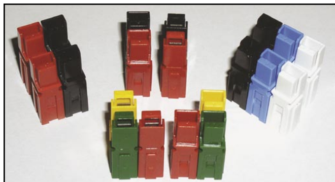
Figure 1 — Notice how these various examples mate. At the top left is a pair of connector bodies in the genderless ARES and RACES configuration.
