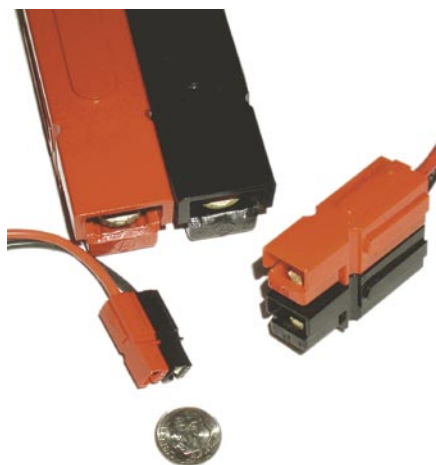
Figure 2 — Here are several sizes of Powerpole connector assemblies. We use the smaller ones rated for cool running at 45 A continuous with 10 gauge wire. The big ones are rated for 250 A, continuous.
