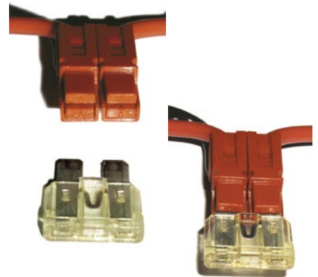
Figure 8 — Anderson Powerpoles rigged as an automotive ATC/ATO fuse holder. See the text for an explanation of how to make this fuse holder.
