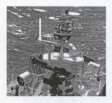
Boats & Ships also have lower powered radar systems, but they are still hazardous if you find yourself in its path. There is no safe way to approach a rotating radar antenna. De-energize the system by having the ship's radar officer do so. This antenna is the radar antenna on Fire Boat 2. No maintenance should be done near this antenna when it is rotating.
