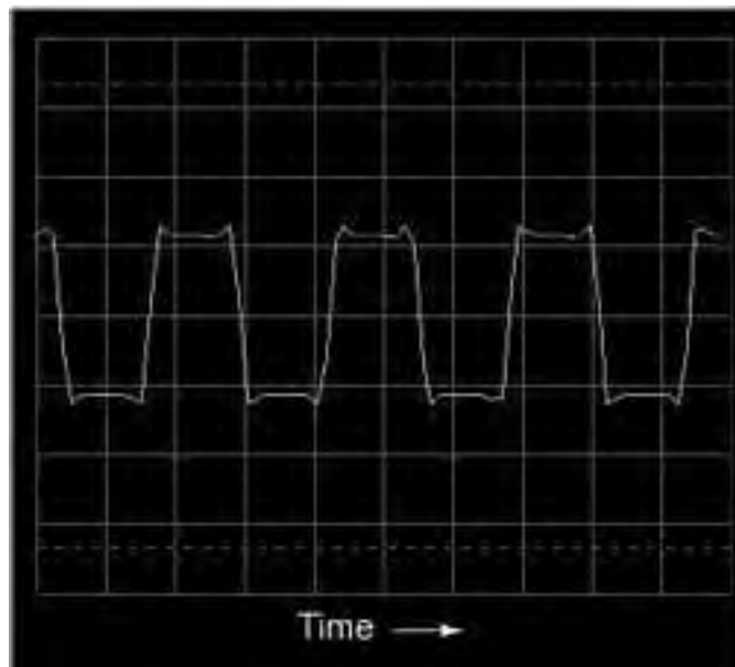
Figure 7.31: Oscilloscope time-domain display of a square wave
