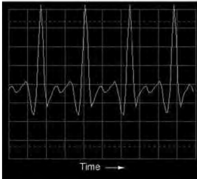
Figure 7.27: Oscilloscope display: waveshape of a trumpet tone.
