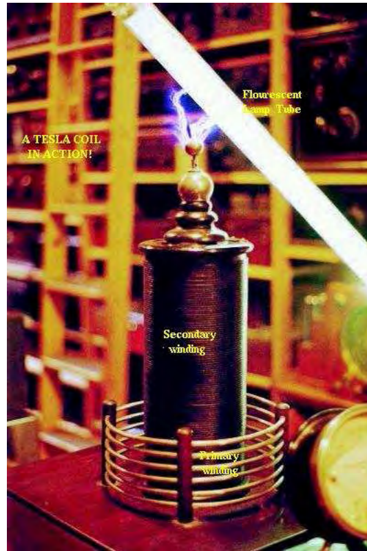
Figure 9.54: High voltage high frequency discharge from Tesla coil.
