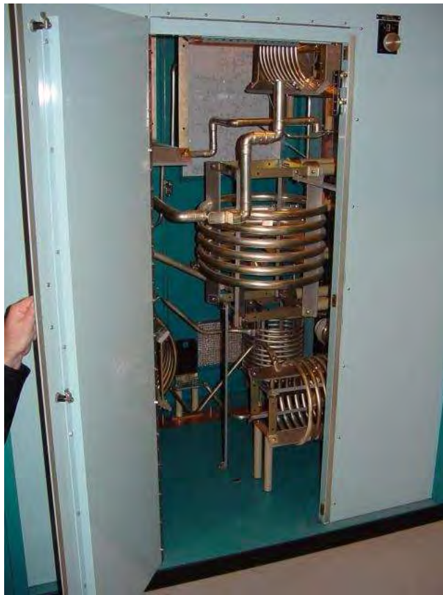
Figure 3.18: High power inductors formed from hollow tubes.
