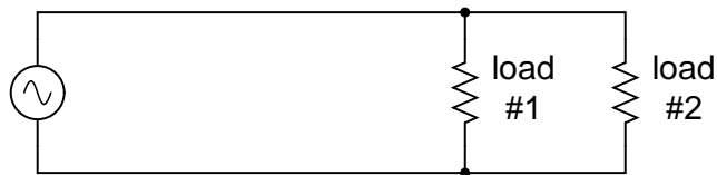
Figure 10.1: Single phase power system schematic diagram shows little about the wiring of a practical power circuit.
