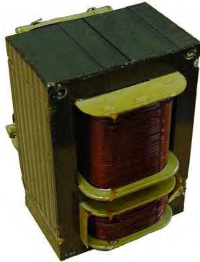
Figure 9.10: Example of a gas-discharge lighting transformer.
